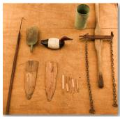
hand-pile driver used to put in poles for pound nets.
